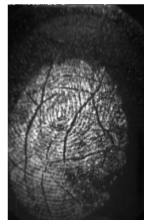
Bad Image: An image where the crackles & displacement of the fingerprint core decries it unrecognizable.
